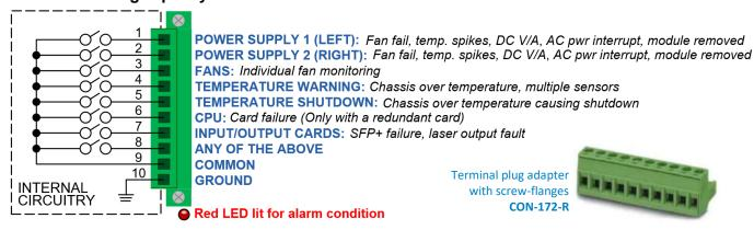
All fan speeds are monitored and any that do not meet specification will cause an alarm condition.
