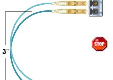
Warning! Minimum bend diameter must be no less than 3". Be careful not to kink or pinch the fiber when using ties.
