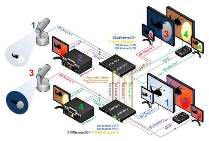
**2.8.2 Four SDI Video Sources,** of which two each are connected to a **T-4200 Chassis** housing two **STM Transceiver Modules**, extending video and peripheral signals, via eight fiber optic cables, to another **T-4200 Chassis** equipped with two more **STM Transceiver Modules**. Each STM TR extends one SDI video IN signal to two SDI video OUT ports. Four separate workstations display dual SDI video outputs from each of the four, single SDI video signals.
