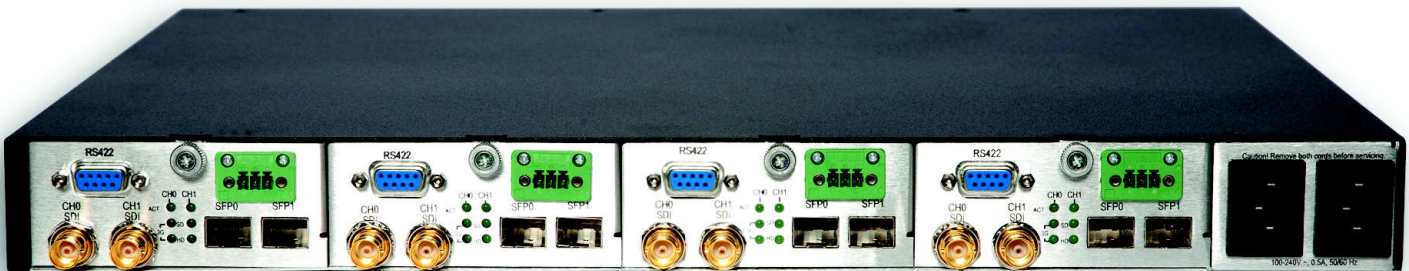
Back View of SDI Xtreme 3G+ Rack Mount Unit - All modules are hot-swappable
