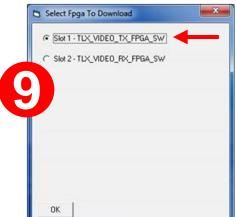
**STEP 9:** You will see a window similar to this, depending on how many slots in the chassis are occupied (2 in this example). As shown, there is one firmware option for each of the TLX Video modules.
