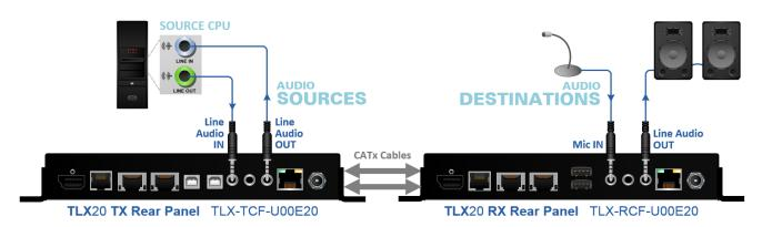
Standard TLX Extender Audio Line In/Out Configuration
