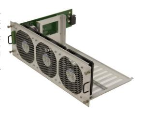
**ALARMS:** The Fan Tray is equipped with an annunciator port for system alarms that can be configured to trigger an external control system. The dry alarm contacts are *Normally Closed* when unpowered, *Normally Open* when powered (OK condition) and *Closed* for an alarm condition. **Maximum switching capacity is 2A at 12V.**
