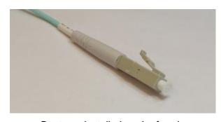
Dust cap installed on the ferrule.
