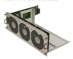
The TLX320 uses 3 DC fans located in one modular, hotswappable fan tray designed for easy replacement without interrupting system functionality. The Fan Tray introduces air into the chassis through air baffles within the chassis. This cools the vertically mounted I/O Cards, the Controller Cards and the backplane.
