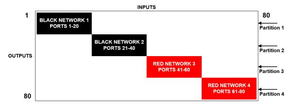
Four partitions set up for secure routing and extension applications. Signals are only capable of transmitting and receiving within a single partition and not across partitions
