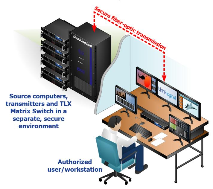
Thinklogical's TLX, VX and MX Matrix Switches use two methods for secure routing. One is known as **Restricted Switching** and the other is known as **Partitioning**. These methods can be deployed singularly or jointly, depending on security requirements.
